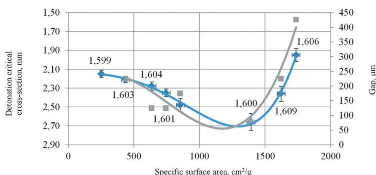
Fig. 1. Overlaying curves illustrating changes in detonability determined by the wedge and air-gap methods
