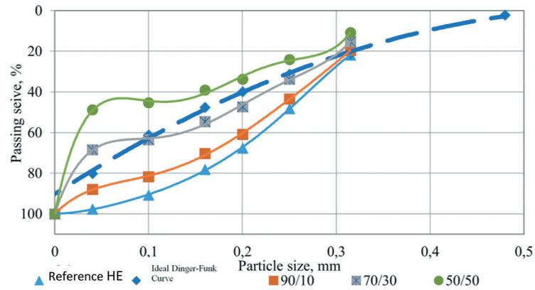
Fig. 2. Ideal Dinger-Funk particle size distribution curve (dashed line) and particle size distribution curves for the reference HE and the bimodal compositions with ratios 90/10, 70/30, and 50/50
